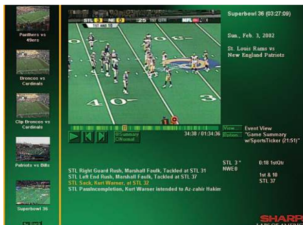
[FIG9] A screen shot from a Sharp prototype system for American football. The game statistics extracted from the SportsTicker data feed are shown to the right and lower-right corner of the main window. Directly below the window is a scrolling textual description of the game, with each line corresponding to a play and the line in golden font corresponding to the current play being viewed.
