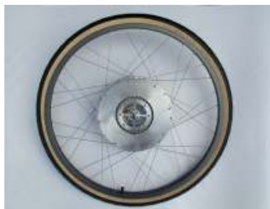
Figure 2: Front wheel with integrated motor
