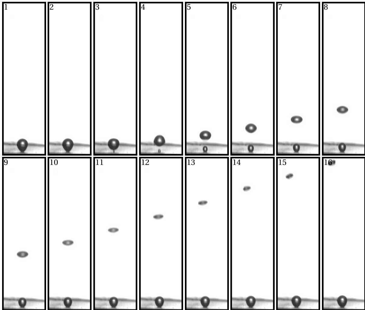
Figure 5.70: Photos of a typical bubble rise, at a wall superheat of \Delta T_W \approx 3.5 K. Time difference between two photos is \Delta t = 2.5 ms. Physical height represented is \Delta z \approx 14 mm.
