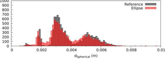
Figure 13: Bubble size histograms for the test case at 5 % gas fraction.
