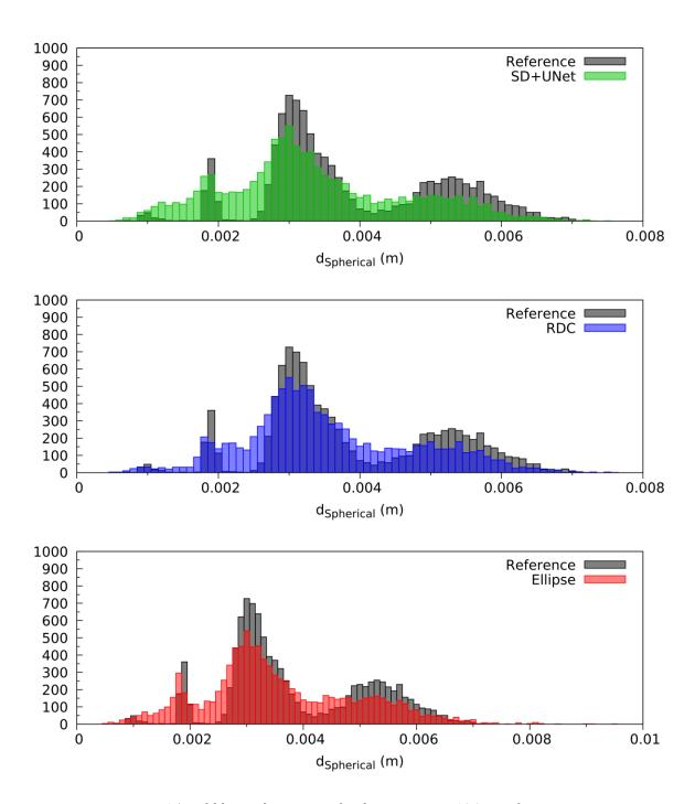
Figure 15: Bubble size histograms for the test case at 10 % gas fraction.
