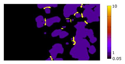
Figure 3: Weight map for the loss function to train the segmentation between bubbles and background (UNetL3) for the example given in Figure 2.
