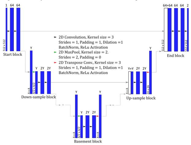
Figure 1: UNet architecture and used parameters. Y refers to the number of filters and A to the input dimension for the respective layer, where Y increases and A decreases up to the basement block. Correspondingly, the Basement block of UNetL3 has Y=256 and A=128, while the UNetL5 has Y=1024 and A=32.
