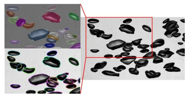
Figure 8: Generated example image for gas volume fraction of 5 % (right) with the segmentation mask from StarDist+UNet (top left) and the overlapping outlines corrected with the RDC method (bottom left).
