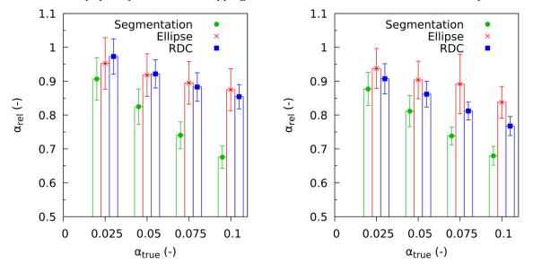
Figure 9: Gas volume fraction results with respect to the ground truth gas volume fraction using ideal segmentation (left) and the combined SD+UNet segmentation (right).
