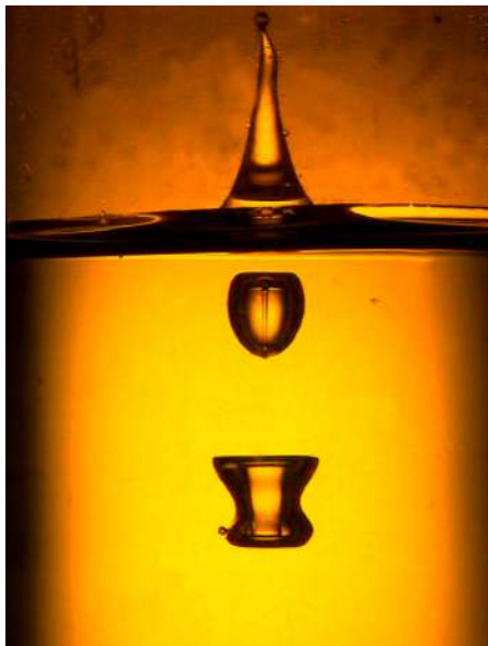
FIG. 11. Comparable process to Fig. 10 at a later stage. Two jets have developed at the singularity: one upward and one downward into the bubble. This photo has been taken from Ref. [14].
