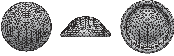
Fig. 16. Top, side and bottom views of the equilibrated configurations of an adhering spherical shell when the sets of the scaled elastic constants are (C_s/\epsilon, C_b/\epsilon) = (30, 1) .
