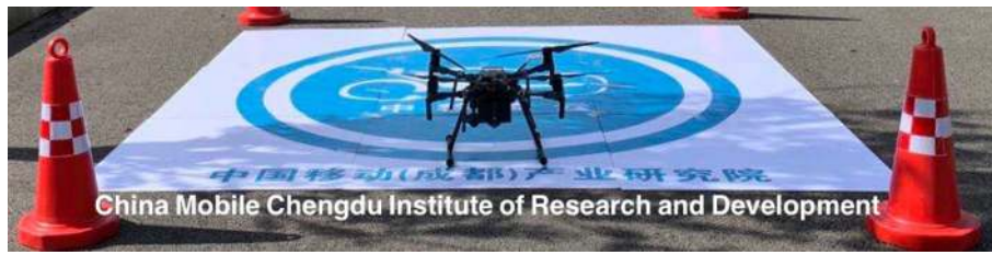
Fig. 4 DJI M210 UAV equipped with a 5G communication module provided by China Mobile Chengdu Institute of Research and Development
