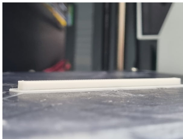
Figure 8. The printed target model (stick) on the build plate using the Peltier module.
