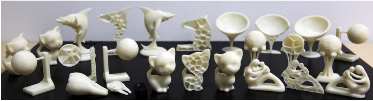
Figure 10: We build-to-last and 3D print our models as well as their hollowed honeycomb-like interiors. A standard key is as the size reference.
