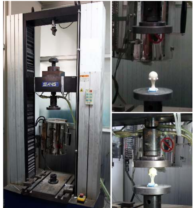
Figure 11: Compression tests using a universal testing machine.
