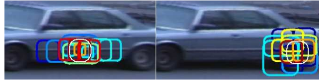
Figure 3: Patch Correlations . On each image, the patches most correlated with the white-circled patch are shown. Notice that in the left image, where the patch sits in an area with a highly visible horizontal structure, the most correlated patches all lie along the horizontal features. Contrast this with the right image, showing correlation of patches with a patch sitting on a wheel, where the most correlated patches are those that strictly overlap the white-circled patch.
