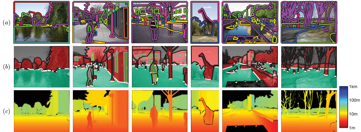
Figure 5. System outputs. (a) Input image and object labels. (b) Polygon and edge types (see Figure 2 for color key). (c) Depth maps (in meters) produced by our system, with a legend for the depths (in log-scale) shown at right.
