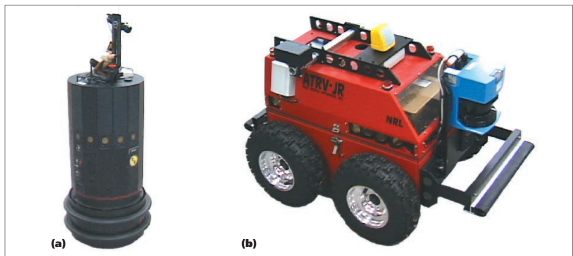
Figure 1. We implemented our interface on a team of (a) Nomad 200 and (b) Real World Interface ATRV-Jr. robots.
