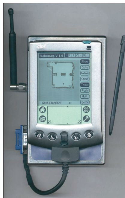
Figure 3. Users can enter commands through a Palm Pilot, which presents a map of the robot's environment.
