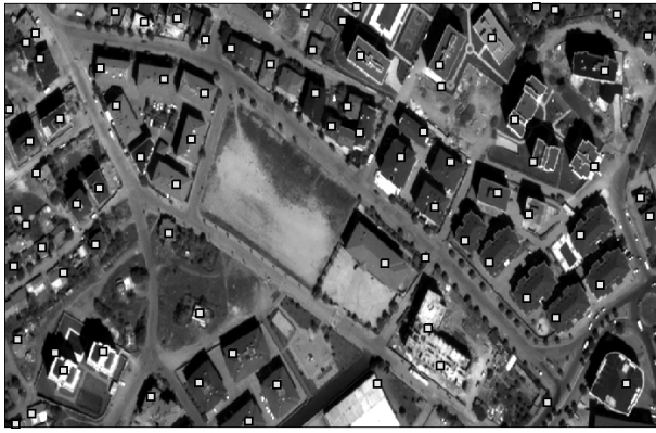
Fig. 10. Building detection results from the residential area using corner points.
