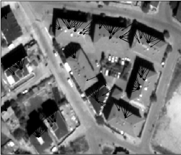
Fig. 6. Kernel directions using the shadow pixels extracted for the first test image.
