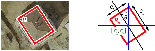
Fig. 1. Definition of the rectangle parameters
