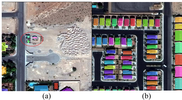
Figure 5. Extraction of special types of buildings: (a) small buildings in red circle, and (b) multiple buildings in close distance. Different colors are used to represent different building footprints extracted.
