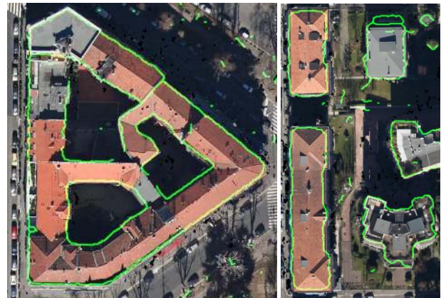
Figure 11. Examples of the extracted building footprints (skeletonized outlines) overlaid onto the true orthophoto.
