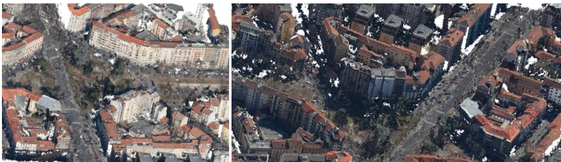
Figure 2. Example of a dense point cloud from oblique images.
