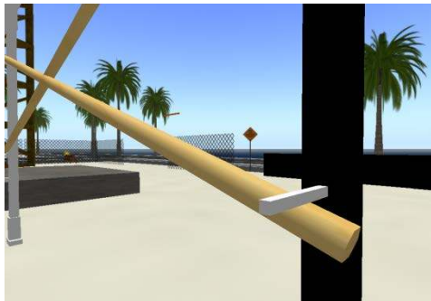
FIG. 8: Scaffold training- Dislocated component and missing safety pin (left image)
