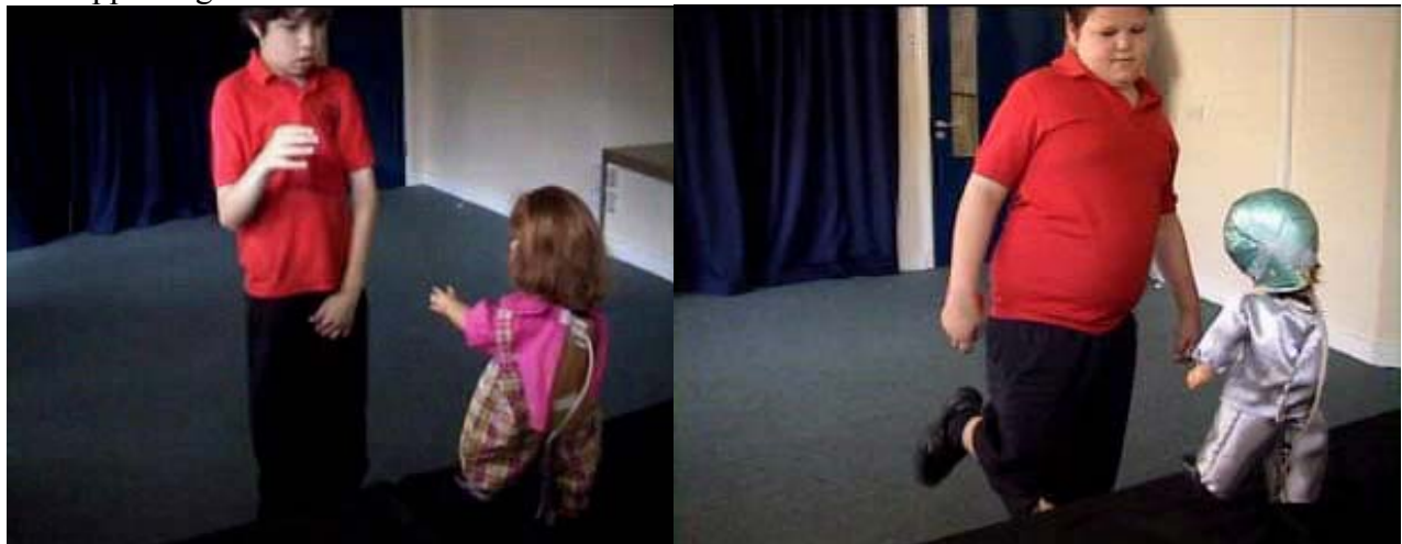
Figure 5: The robot in its two different appearances – pretty doll (left) and plain (right). Two children playing a limb-to-limb imitation game involving legs, head and arms. In this work, Robota’s mirroring the motion is working in a ‘puppeteering mode’, i.e. as a remote controlled robot where the experimenter picks up subtle movements of the children and responds with contingent movements of Robota’s limbs and head.
