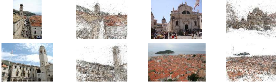
(a) Dubrovnik: Four different views and associated images from the largest connected component. Note that the component captures the entire old city, with both street-level and roof-top detail. The reconstruction consists of 4,585 images and 2,662,981 3D points with 11,839,682 observed features.
