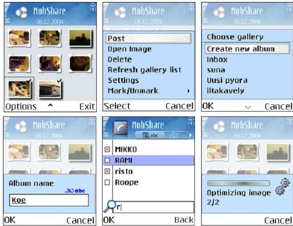
Figure 1. The sharing of pictures in the MobShare phone client. First the pictures are selected for posting, and then a new gallery/album is created for the selected pictures. The gallery is named and the recipients are selected. In the end the pictures are optimized and uploaded to the web server.
