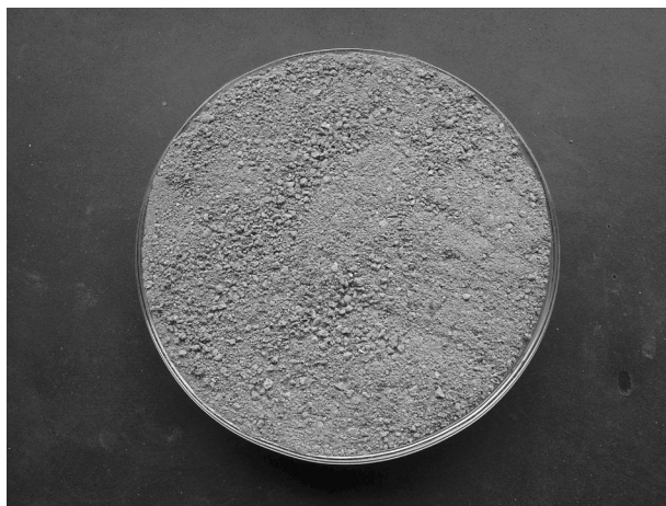
Figure 1. Soil sample in dish prepared for spectra measurements
