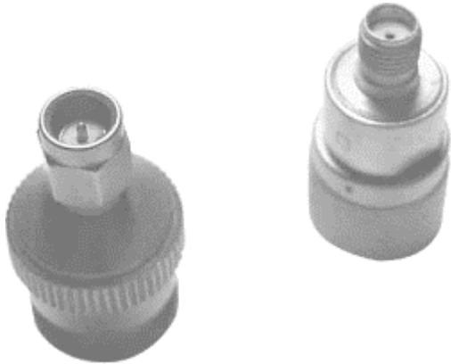
Figure 6-16. SMA: Sub-Miniature connector, variation A
