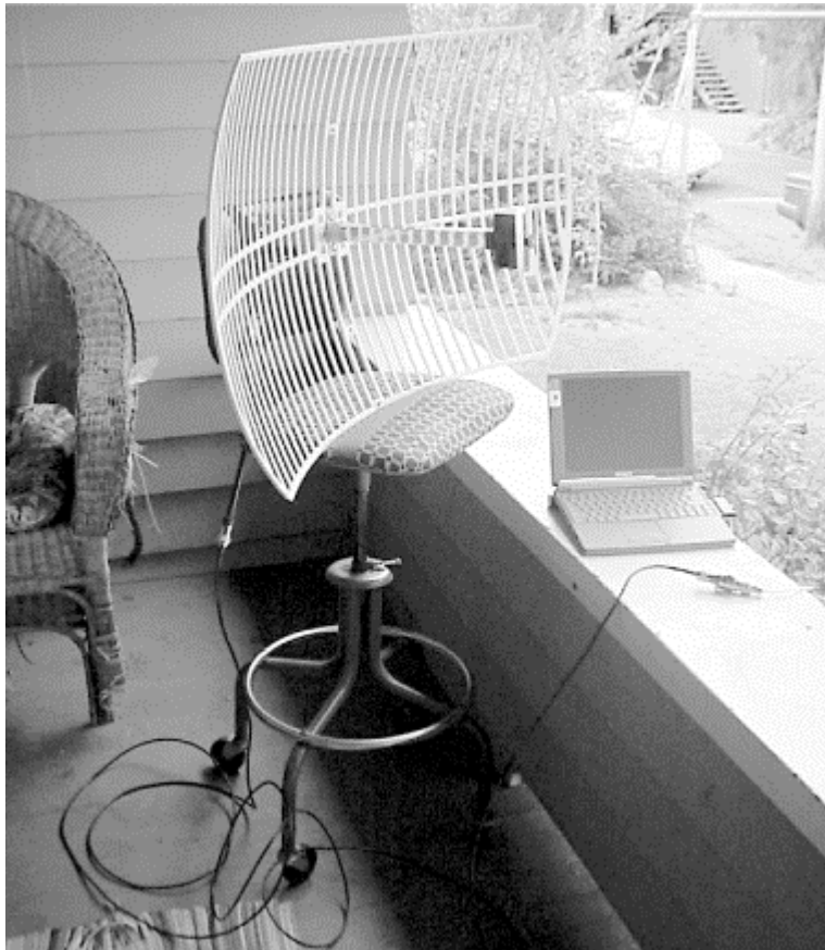
Figure 6-11. A 24dB parabolic dish
