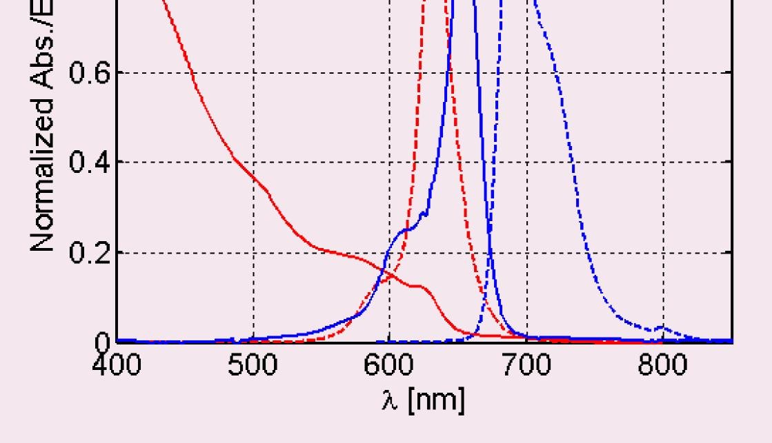
Absorption and emission spectra of CdSe/CdS/ZnS core/shell/shell quantum dots and SQ02 dye molecules . There is a large overlap between emission spectrum of the QDs and absorption spectrum of dye molecules.
