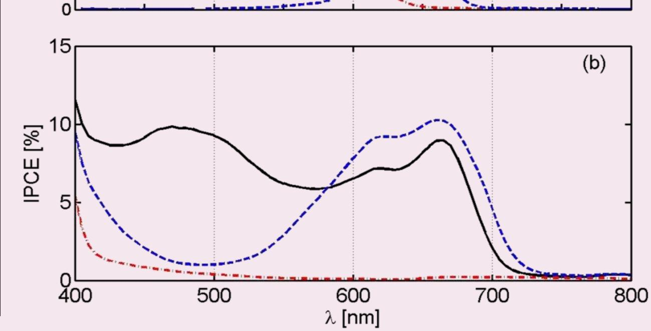
A cell consisting of QDs only (dashdotted red curve); a cell containing only dye molecules (dashed blue curve); the complete cell including the QD antenna layer and the dye molecules (solid black curve).
