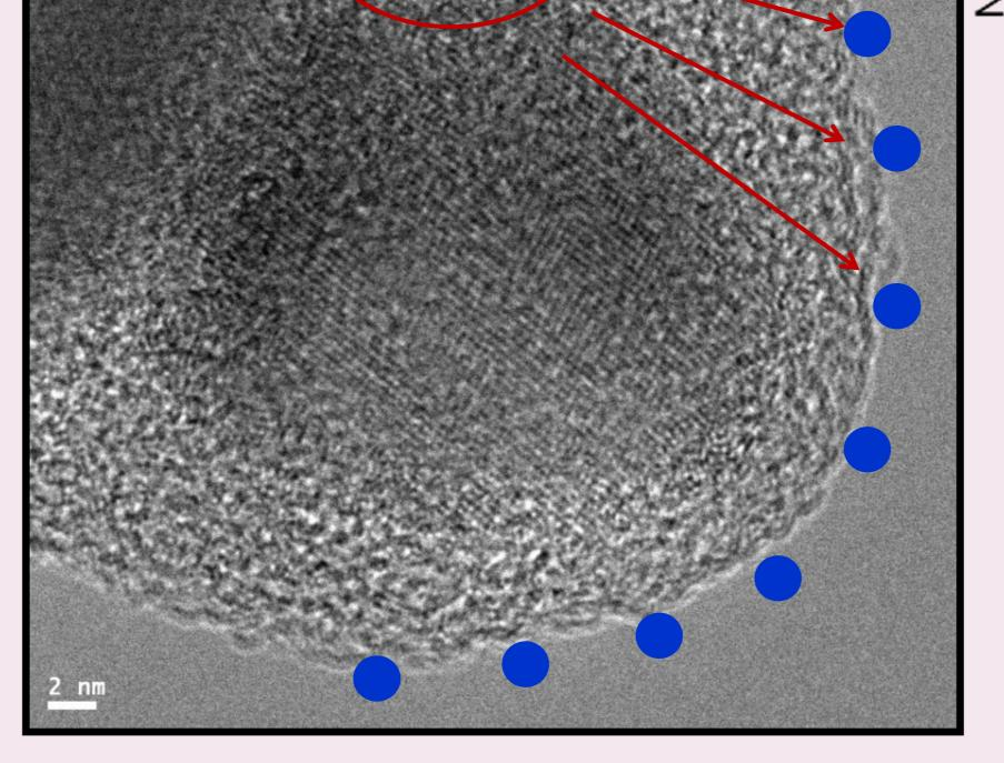
HR-TEM image showing wurtzite structure of CdSe/CdS/ZnS QD bound to the nc-TiO<sub>2</sub> and fully covered by an amorphous  $TiO_2$  coating
