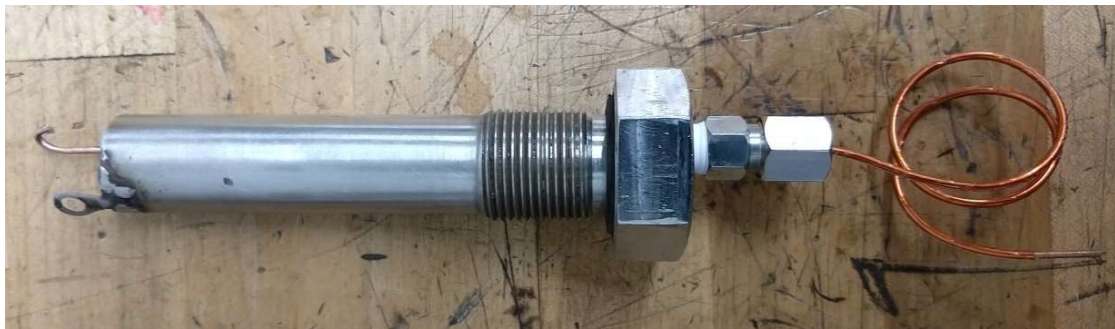
Figure 8 Custom sample holder used to load samples into the test vessel.
