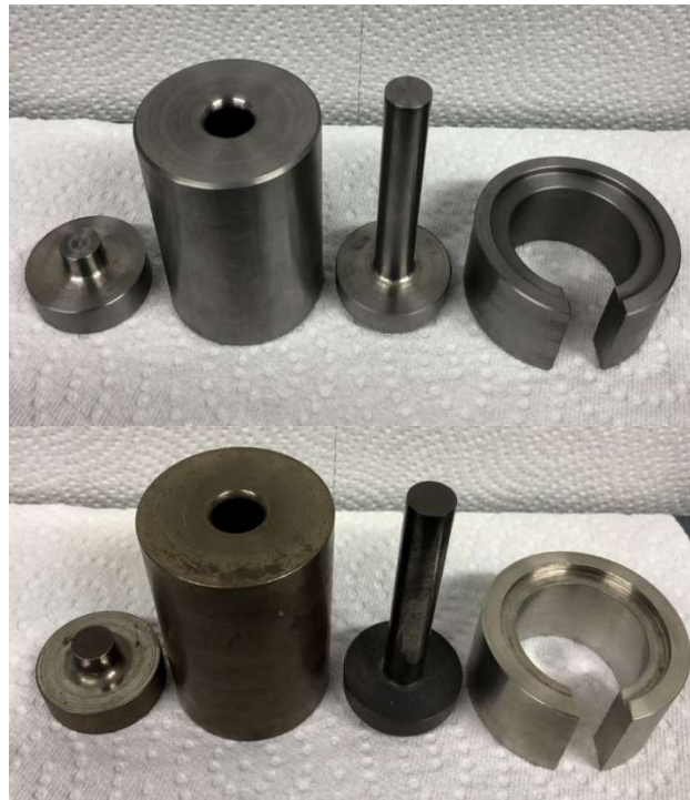
Figure 4 (top) Pellet punch assembly prior to heat treatment. (bottom) Pellet punch assembly after heat treatment.
