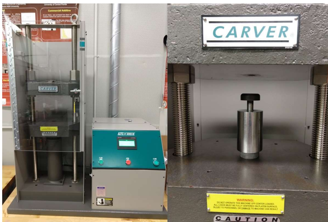
Figure 5 (left) Carver M-NE3890 programmable hydraulic press. (right) Pellet punch assembly loaded into the Carver hydraulic press.
