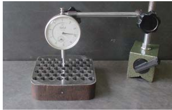
Figure 3. Illustration of measurement of the burr height at the end of the holes of a sample.
