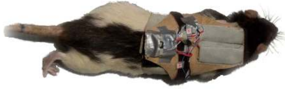
Figure 1. A Norway rat is wearing a sensor jacket. While this attachment is sufficient for lab environments, outside deployments will require more robust attachment.
