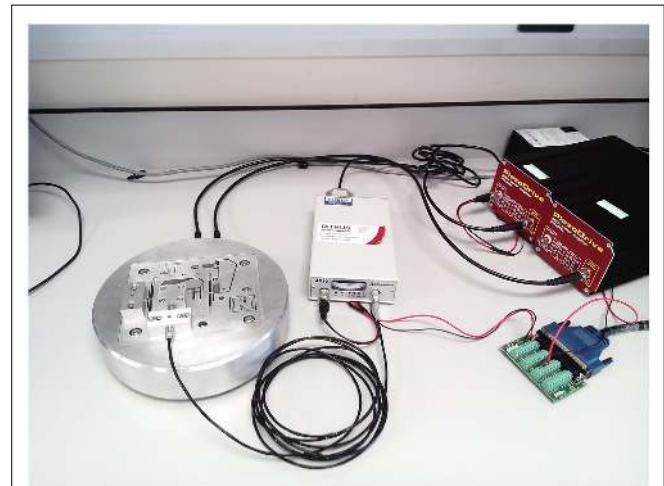
FIGURE 3 | A two-axis serial kinematic nanopositioner, designed at the EasyLab, University of Nevada, Reno, driven by two PiezoDrive 200V Linear amplifiers, with position measured by a Microsense 4810 capacitive sensor.
