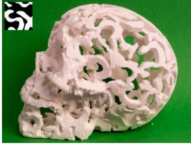
Figure 14: Result printed on a ZCorp 450. On this type of machines the printed objects are very fragile and have to be extracted from the powder bed before dipping into cyanoacrylate. Our thin patterns nevertheless print successfully.
