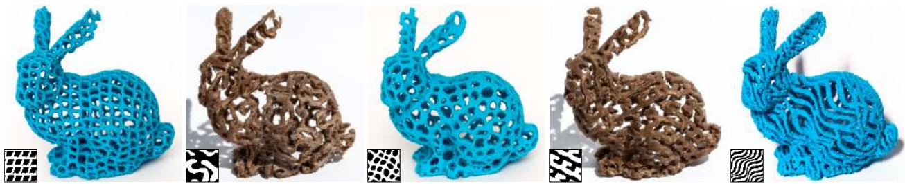
Figure 1: Our by-example pattern synthesis algorithm produces structurally sound patterns along the surface of an object, resembling the input exemplar. The reinforcements are integrated within the pattern, by a joint optimization of appearance and structural properties. Top: The Stanford bunny with a variety of synthesized patterns. Bottom: Example patterns. These objects are printed in ABS plastic on low-cost filament printers, using a dense support. The patterns are fully connected and survived the cleaning process thanks to their reinforced structure. Yet, the reinforcements are inconspicuous as they seamlessly blend within the appearance.
