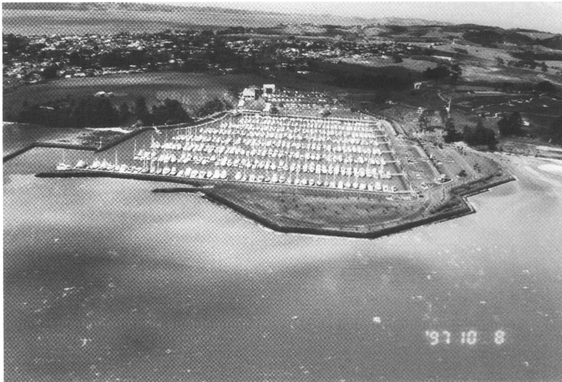
Figure 13. Turbidity and high suspended load from the estuarine turbid fringe and from the stream adjacent (to the right) of the marina flowing under the influence of southwesterly winds into the marina approach channel, where muddy deposition occurs. Such "natural" turbidity is higher than measured at the monitoring sites related to the dredging.
