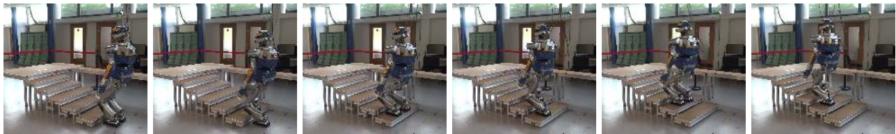
Fig. 13: Snapshots of the motion for the 10cm stairs, the complete motion is shown in the companion video.
