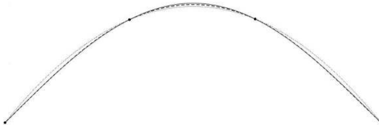
Figure 3: Approximation of a sine curve (solid) by a C^2 cubic spline (dotted) interpolating discrete points, and by a C^2 PH quintic spline (dashed) interpolating both points and segment arc lengths. The data points correspond to the parameter values t = 0, \frac{1}{3}\pi, \frac{2}{3}\pi, \pi on the curve \mathbf{r}(t) = (t, \sin t, 0) .
