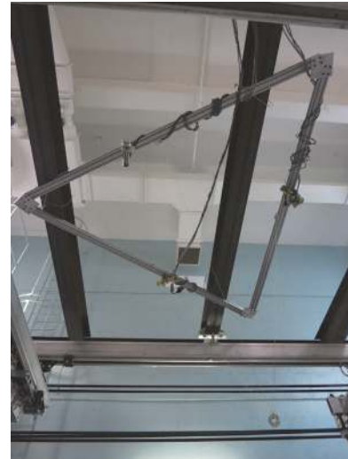
Fig. 8 Prototype of a 3-cable 3-dof CSPM developed at Laval University for the performance of dynamic trajectories that extend beyond the static workspace.
