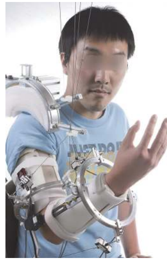
Fig. 4 Prototype of CAREX, a cable-driven arm exoskeleton for neural rehabilitation developed at Columbia University (courtesy of Professor Sunil Agrawal, Columbia University).
