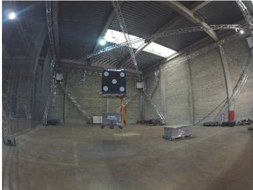
Fig. 7 Prototype of the CoGiRo, an 8-cable 6-dof CDDM for material handling developed by LIRMM and Tecnia (courtesy of Dr. Marc Gouttefarde, LIRMM).
