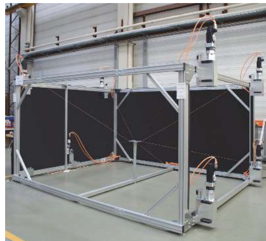
Fig. 6 Prototype of IPAnema-1, an 8-cable 6-dof CDDPM for material handling developed at the Fraunhofer Institute (courtesy of Dr. Andreas Pott, Fraunhofer IPA).
