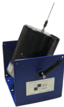
Fig. A.1 The electrodynamic vibration shaker
