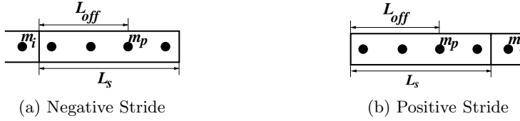
Fig. 3. Cold miss examples along a spatial reuse vector when a memory line boundary is crossed. If m_p is the array element accessed in the previous iteration, the access of array element m_i in the current iteration will result in a cold miss.
