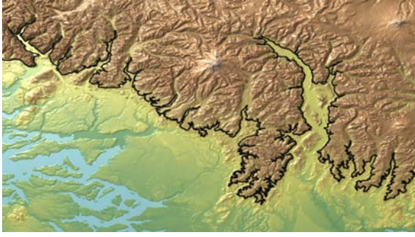
Figure 5: Puget Sound contour line: This image shows a contour line (in black) extracted from an unstructured terrain model of the Puget Sound. The terrain is simplified down to 143M triangles. We extracted the largest component (223K edges) of the level set at 500 meters of elevation. Our cache-oblivious layouts improve the performance of the isocontour extraction algorithm by more than an order of magnitude.
