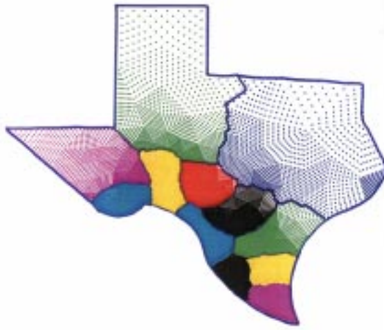
FIG. 4.1. Decomposition of a grid into cache blocks by using the METIS load balancing package.
