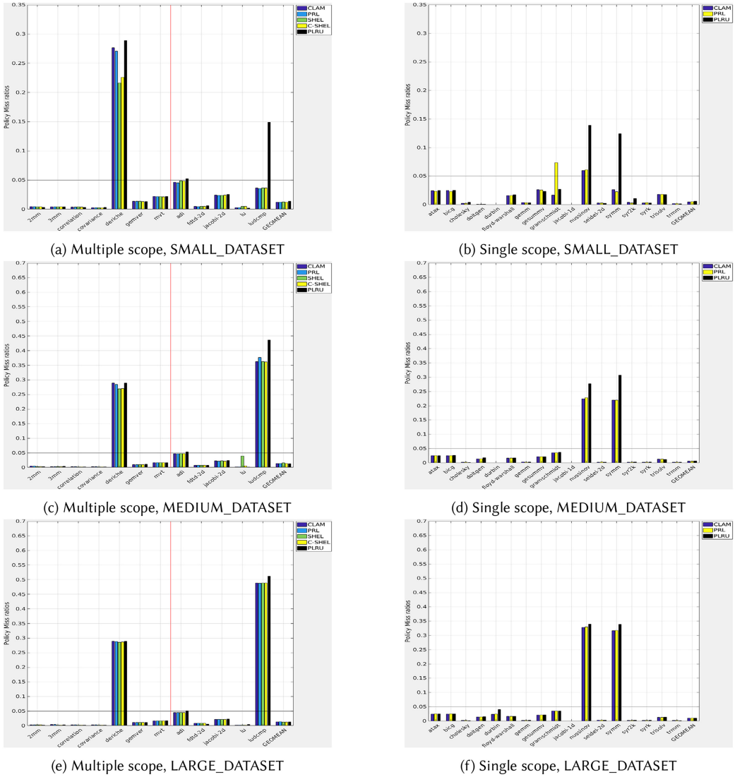
Fig. 7. Miss counts for 12 multi-scope benchmarks (left) and 17 single-scope benchmarks (right) as well as their geometric means after optimized by PLUTO compiler. Lower is better. Values are reported for small (top), medium (middle), and large (bottom) inputs.
