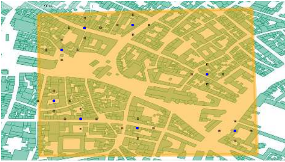
Fig. 1. Considered portion of RAN of the city centre of Ghent (Belgium), composed by 8 macro cell BSs, each supported by 4 micro cell BSs.
