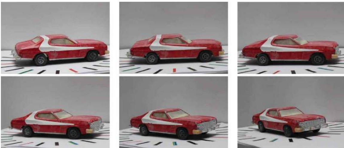
Figure 5. Photos of the model taken with different angle translations with camera at constant height and center of model approximately centered within the frame.
