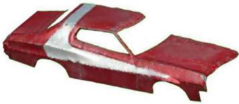
Figure 21. Cleaned triangular mesh of the car body with other parts removed by color segmentation.
