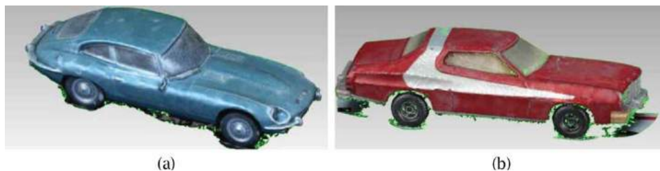
Figure 18. Triangular mesh created for: (a) the E-type model, (b) the Gran Torino model.
