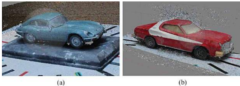
Figure 17. Final dense point clouds on: (a) the E-type model; (b) the Gran Torino model.
