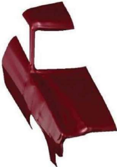
Figure 22. 3D CAD surfaces of body panels generated from the triangular mesh in Fig. 21.
