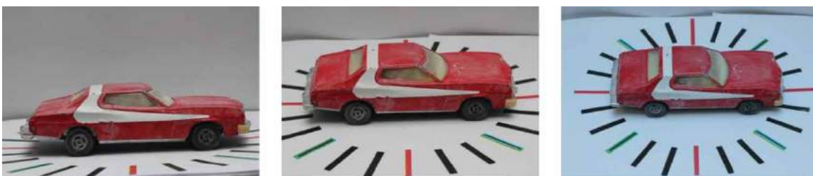
Figure 6. Photos of the model taken for different height translations with camera approximately focused on the center of the model.
