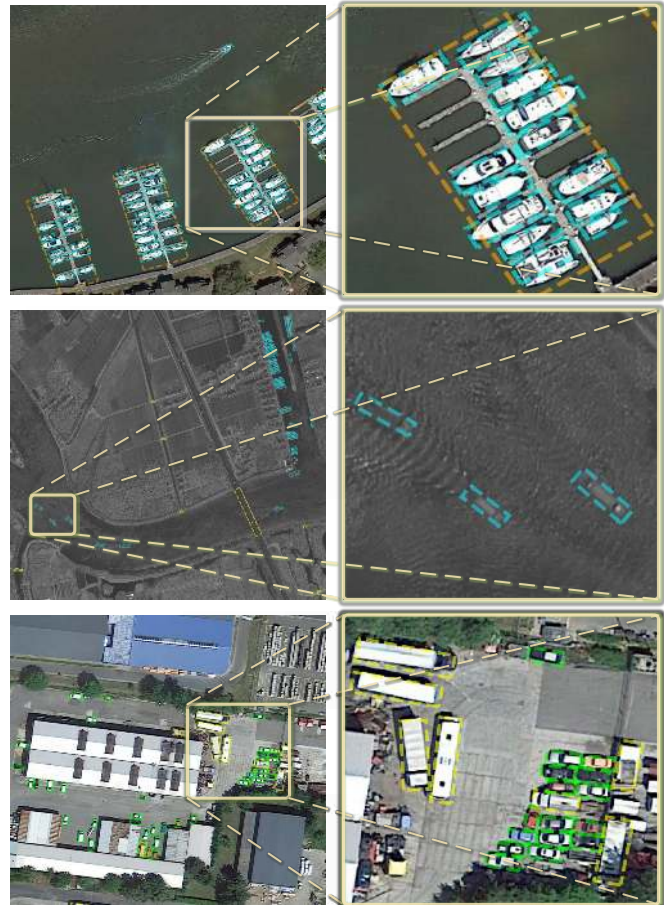
Fig. 1. Illustration of results produced by the proposed CAD-Net for object detection in optical remote sensing imagery: Multi-class objects with different types of image degradation and information loss in colors, contrast and texture are detected and recognized correctly.
