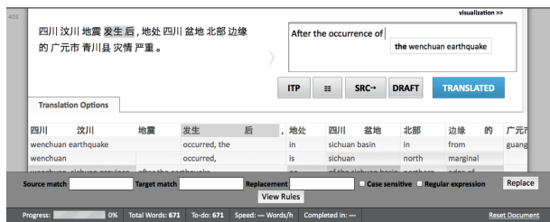
Figure 4: Translation User interface (CASMACAT). The user can see the source sentence (e.g. in Chinese) on the left pane, and can type in or post-edit the translation (e.g. in English) on the right pane.
