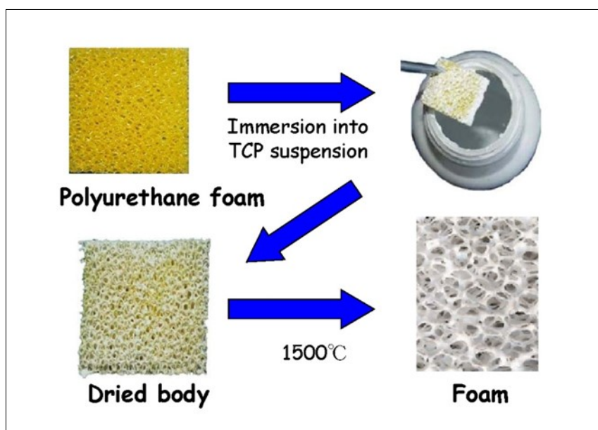
Fig. 5. Photographs of a commercially available porous CaPO 4 scaffolds with different porosity (top) and a method of their production (bottom). For photos, the horizontal field width is 20 mm.
