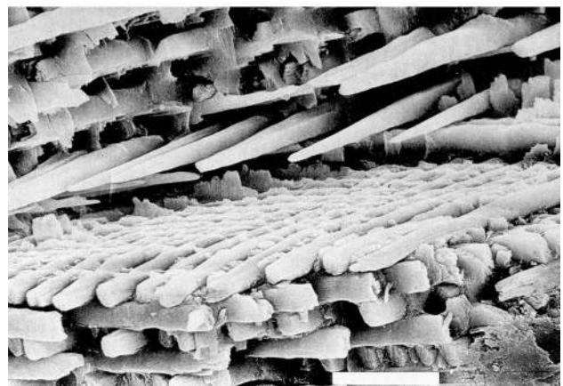
Fig. 15 Top a schematic drawing of a tooth. Other very good graphical sketches of the mammalian tooth structure, including the hierarchical levels, are available in Refs. (Palmer et al. 2008; Meyers et al. 2008). Bottom a scanning electron micrograph of the forming enamel of a continuously growing rat incisor showing ordered rods of \text{CaPO}_4 . Scale bar 10 \mu\text{m} . Reprinted from Ref. (Lowenstam and Weiner 1989) with permission
