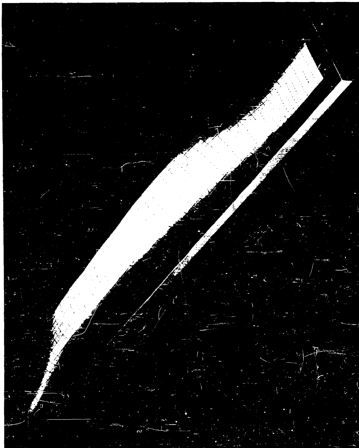
Half-model of a merchant ship hull. This photograph illustrates the manner in which a continuous three-dimensional shape is approximated by plane quadrilateral surface elements. The dots represent the points where velocities and pressures are calculated. (See Section 11.42).
