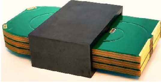
Fig. 6. Constructed 32:4 planar transformer
