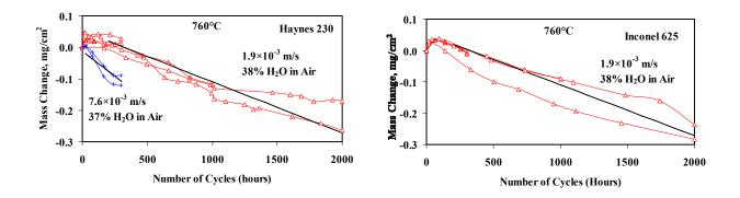
Fig. 4. Cyclic oxidation of Haynes 230 (UNS NO6230)<sup>22</sup> and Inconel 625 (UNS NO6625) at 760°C in moist air. Triangle data points for  $1.9 \times 10^{-3}$  m/s and plus data points for  $7.6 \times 10^{-4}$  m/s. Straight solid lines are the predicted slopes (on a Cr<sub>2</sub>O<sub>3</sub> basis) from reactive evaporation of Cr<sub>2</sub>O<sub>3</sub>(s) to CrO<sub>2</sub>(OH)<sub>2</sub>(g) using the Gindorf<sup>21</sup> data for CrO<sub>2</sub>(OH)<sub>2</sub>(g).
