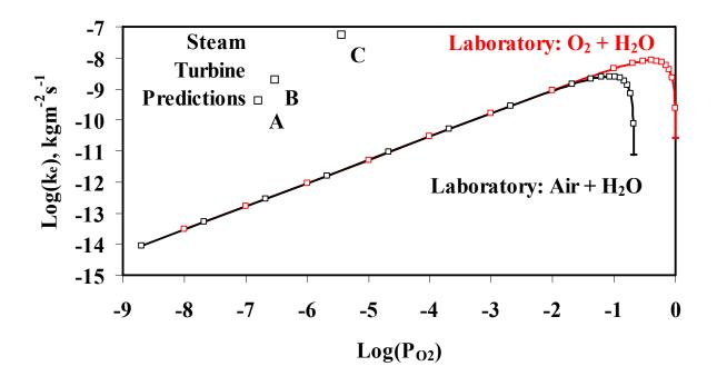
Fig. 7. Predicted evaporation rates for steam turbines (A, B, and C) compared with atmospheric pressure laboratory tests (760°C, u = 0.02 m/s, L = 0.02 m) as a function of the partial pressure of O<sub>2</sub> for tests in either O<sub>2</sub>+H<sub>2</sub>O or Air+H<sub>2</sub>O. "A" is typical for conditions in current power plants, "B" is for current advanced power plants, and "C" is the DOE target conditions (see Table 7).
