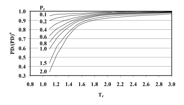
Fig. 1. Reduction of D for dense gases.  $PD/(PD)^{\circ}$  is the ratio of the pressure-diffusivity product at pressure P to the pressure-diffusivity product at atmospheric pressure (both at the same T).  $T_r$  and  $P_r$  are the reduced temperature and pressure and are equal to  $T/T_{critical}$  and  $P/P_{critical}$ . Derived from Slattery and Bird.<sup>12-13</sup>
