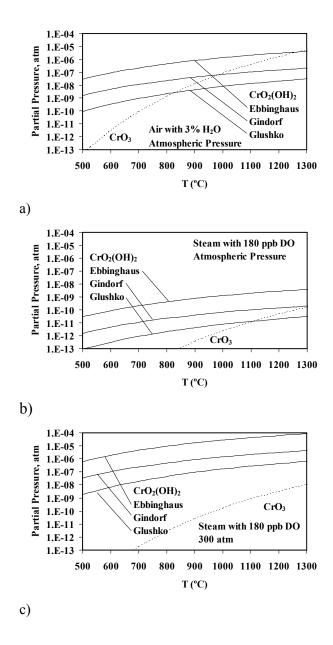
Fig. 2. Partial pressures of  $CrO_3(g)$  and  $CrO_2(OH)_2(g)$  over pure  $Cr_2O_3$  (activity of 1) for a) 3% H<sub>2</sub>O in air at atmospheric pressure, b) steam with 180 ppb DO at atmospheric pressure, and c) steam with 180 ppb DO at 300 atm.
