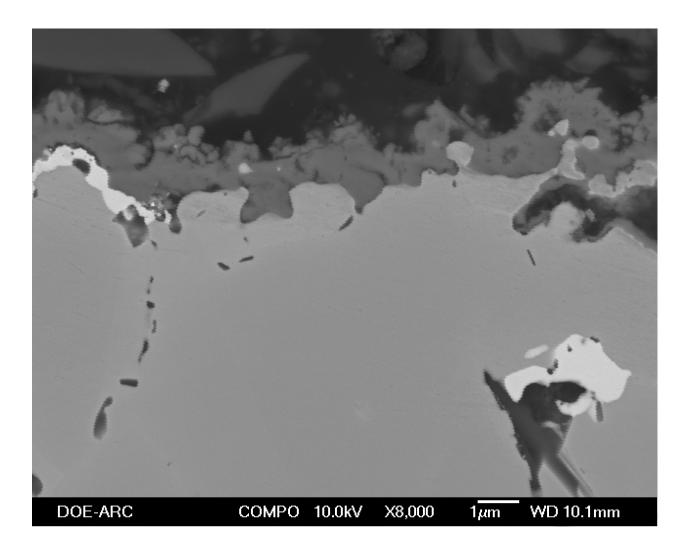
Fig. 5. Micrograph using backscattered electrons of Haynes 230 (UNS NO6230) after exposure at 760°C in moist air for 2000 cycles.<sup>22</sup> The scale is predominately  $Cr_2O_3$ . The bright second phase is W-rich.
