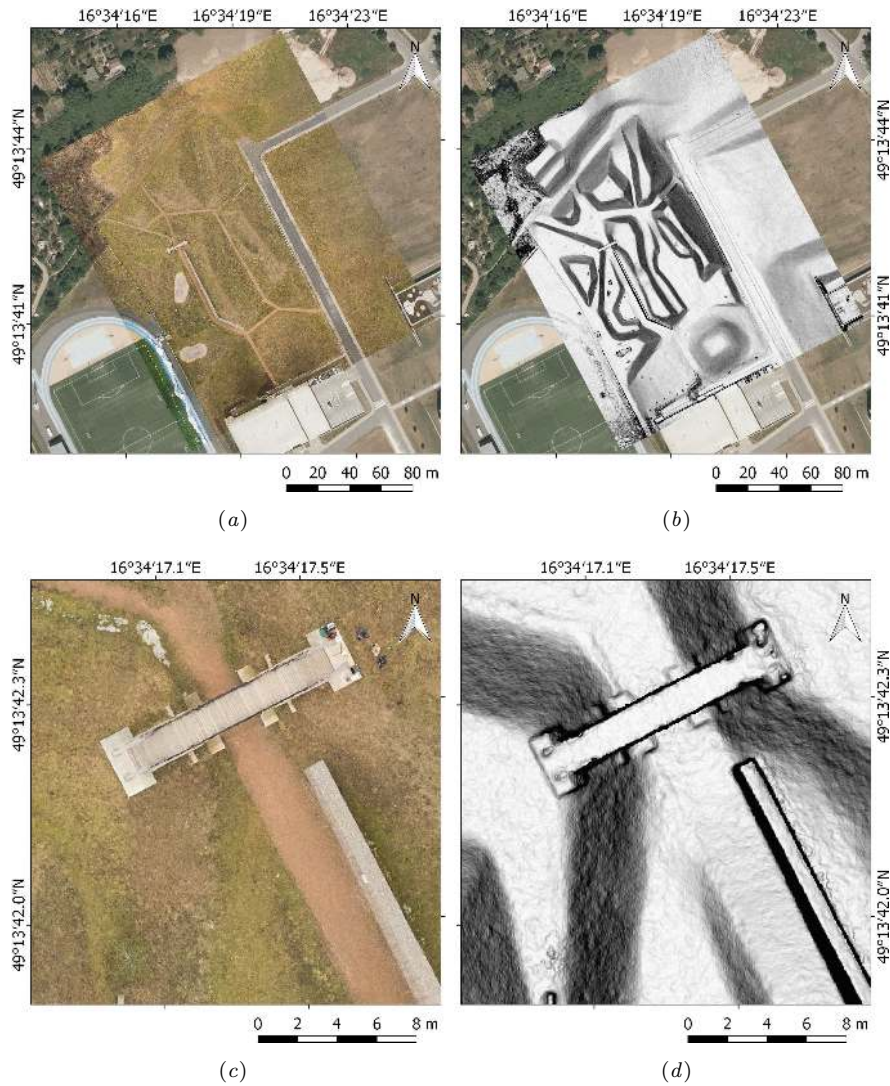
Figure 17. The orthophoto (a) and gradient map (b) created via the presented multi-sensor system as a layer over the orthophoto map adopted from CUZK (2010). Figures (c) and (d) show a detail of the bridge where the base station was located.
