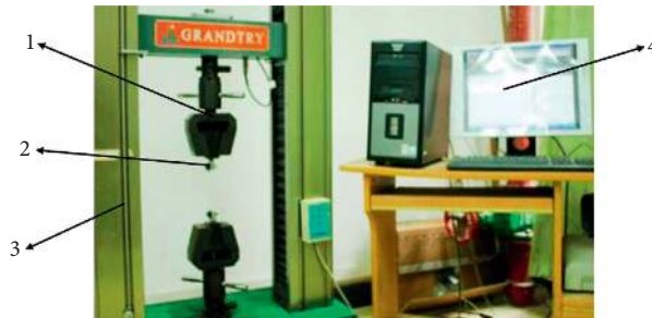
FIGURE 14: Wire elastic modulus test scene. 1. Wire clamp 2. Steel wire 3. Precision electronic universal material testing machine 4. Computer.
