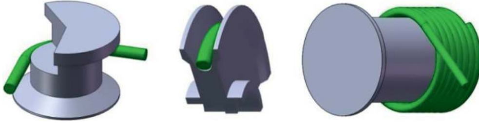
FIGURE 10: The wire rope is in contact with the restraining wheel, pulley, and drum.
