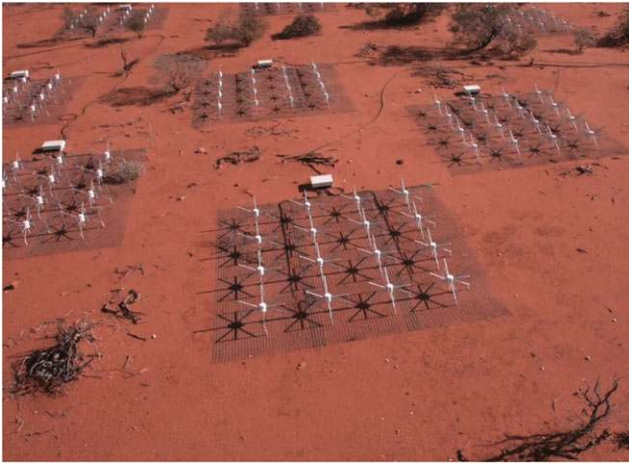
Figure 1. Examples of the MWA's aperture array antenna 'tiles', each comprised of a 4 \times 4 grid of individual bow-tie dipoles (Image credit: MWA Project, Curtin University).
