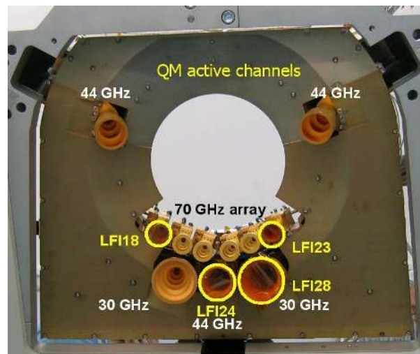
Figure 6. The focal plane unit of the LFI-QM. Circled horns represent the active channels during the test campaign. The other horns in the focal plane are thermally/mechanically representative dummies.
