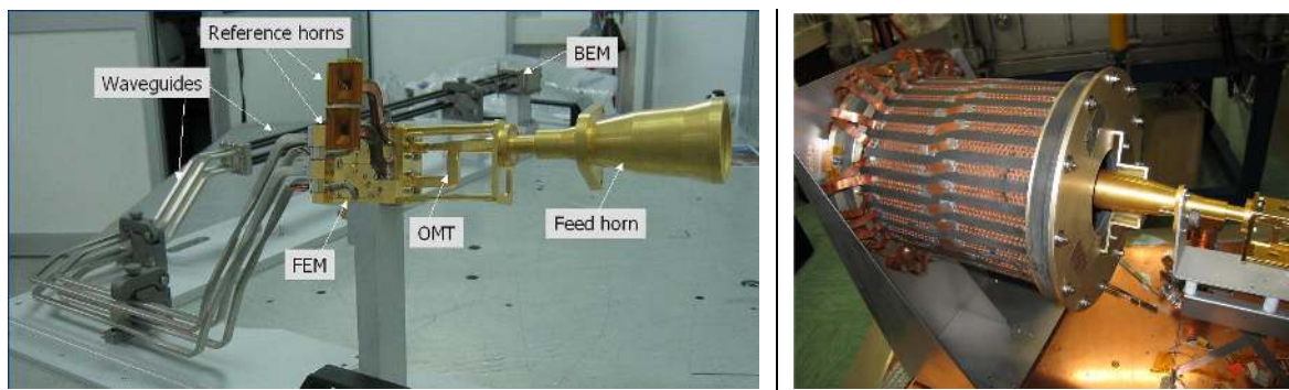
Figure 3. Left: the RCA cryogenic test setup with a 30 GHz receiver before the installation of the sky and reference loads and before being electrically connected and thermally set up for testing. Right: detail of the feed horn pointing in the inner of the sky load.
